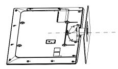
4.Attach the screw from the bottom of the stand to the TV.
